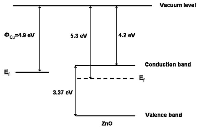
**Fig. 6.** Schematic of the energy band diagrams of copper and ZnO.
