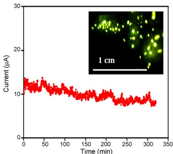
**Fig. 7.** Field emission current stability ( $I-t$ ) plot of the Cu/ZnO nanocomposite film. The inset shows a typical field emission image.
