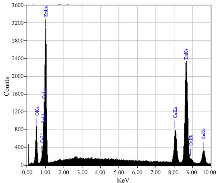
**Fig. 3.** EDS spectrum of the Cu/ZnO nanocomposite film.
