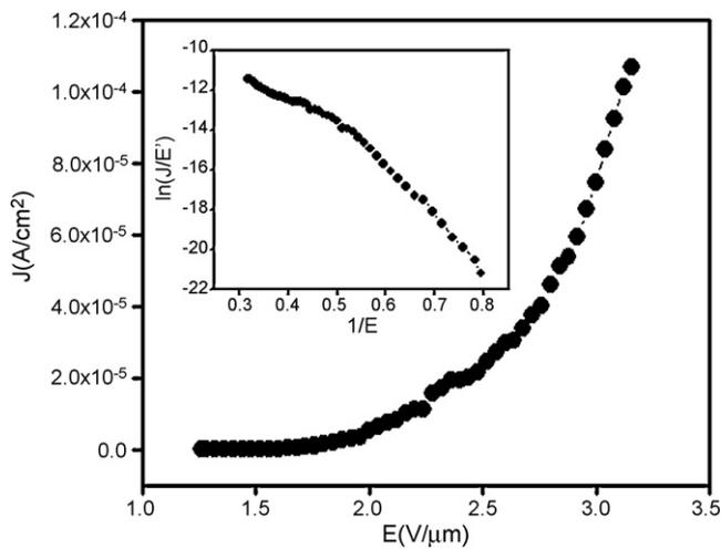
**Fig. 5.** Field emission current density versus applied field ( $J$ - $E$ ) curve of the Cu/ZnO nanocomposite film. The inset depicts the corresponding Fowler-Nordheim (F-N) plot.
