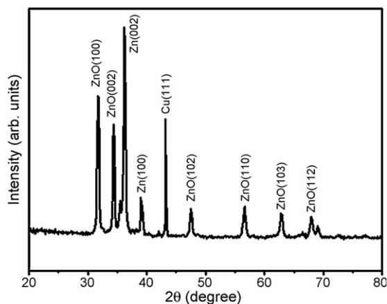
Fig. 1. XRD pattern of Cu/ZnO nanocomposite film.
