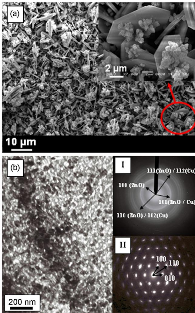
**Fig. 2.** (a) Low and high magnified SEM images and (b) TEM micrograph of the Cu/ZnO nanocomposite film. The inset of TEM micrograph shows two distinct SAED patterns corresponding to the Cu nanoparticles and ZnO sheets (b(I)) and ZnO microsheets (b(II)).
